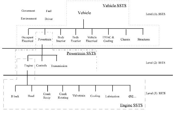
Diagram 1.1-I Powertrain SSTS scope of work
